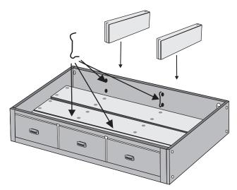
12) To use the bottom bed as a storage drawer, simply remove the mattress and insert the four wire retainers as shown above. Slide the drawer partitions into the wire retainers down the grooves on the partitions.
