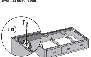
Attach casters to bottom of bed using two screws for each caster (G). Notice the casters are located on the inside of each rail.
