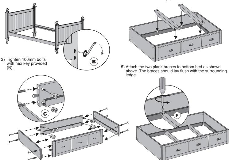
3) Attach the two bottom bed end panels to the front and back panels. Use the 60 mm bolts and barrel nuts as shown in the diagram(C).
