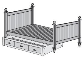
11) Roll the lower bed under the upper bed. Now use the hex key to re-tighten all bolts so that the bed assembly is rigid. It may be necessary to re-tighten bolts after wood has acclimated to your weather region. You are now ready to enjoy your trundle bed.
