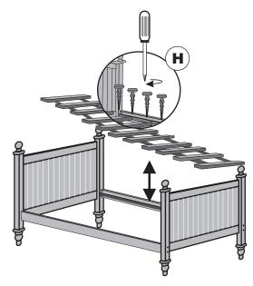
10) Unroll the slat bundle (strap side down) and spread out from end to end of bed. Now attach each slat to the side rail with the 32 screws provided (H).
