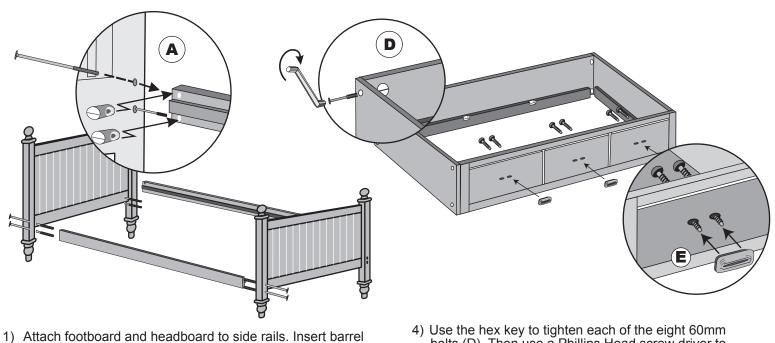
Attach footboard and headboard to side rails. Insert barrel nuts into side rails. Insert 100mm bolts through end boards and into barrel nuts (A). 4) Use the hex key to tighten each of the eight 60mm bolts (D). Then use a Phillips Head screw driver to attach the trundle handles to the front panel using six 35mm small bolts (E).
