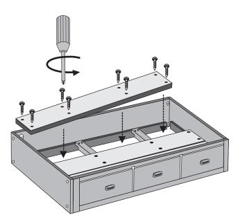
9) Now flip the lower bed back over and lay the three bottom planks into the bed. The top side of the planks will have countersunk holes for the screws. Insert and tighten the eight screws on each plank.
