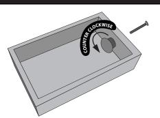
Remove the knob from the inside of the drawer by holding the screw in place and turning the knob counter clockwise.
