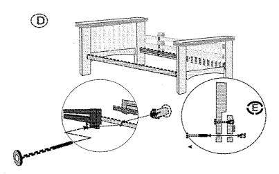
4) Attach both the long and the short safety rails to the the side rails of the upper bunk using eight 50 mm bolts and eight propel nuts (See Diagrams D & E). The long rail will be on the side of the bunk which is opposite the ladder. The short rail will be used on the side of the bunk accessed by the ladder.
