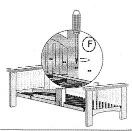
6) Attach slats to side rail ledge with slat screws using a phillips head screwdriver (See Diagram F). A power screwdriver comes in handy here.
