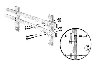
Attach the two long safety rails to the unassembled upright supports using eight 50 mm bolts and eight propel nuts. Tighten with hex key(See Diagrams C).
