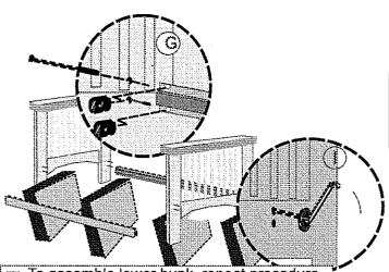
7) To assemble lower bunk, repeat procedure used for upper bunk using taller end boards. (See Diagram G). Tighten 100mm bolts to barrel nuts with hex key (See Diagram I).
