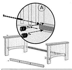
To assemble upper bunk, attach short end boards to upper bunk side rails. The side rails used on upper bunk have predrilled holes for safety rail attachment. Insert barrel nuts into side rails. Insert 100mm bolts through endboards and into barrel nuts (See Diagram A).
