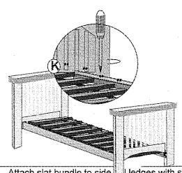
Attach slat bundle to side ledges with slat screws using a phillips head screwdriver. A power screwdriver comes in handy here (See Diagram K).
