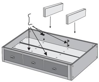
12) To use the bottom bed as a storage drawer, simply remove the mattress and insert the four wire retainers as shown. Slide the drawer partitions into the wire retainers down the grooves on the partitions.
