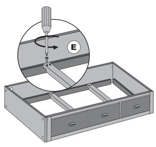
6) Insert the eight large wood screws into the plank braces. Fasten the screws using a phillips head screwdriver (See Diagram E).
