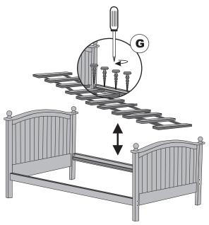
10) Unroll the slat bundle (strap side down) and spread out from end to end of bed. Now attach each slat to the side rail with the 32 screws provided (See
