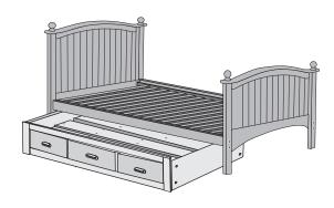
11) Roll the lower bed under the upper bed. Now use the hex key to re-tighten all bolts so that the bed assembly is rigid. It may be necessary to re-tighten bed after wood has acclimated to your weather region. You are now ready to enjoy your trundle bed.
