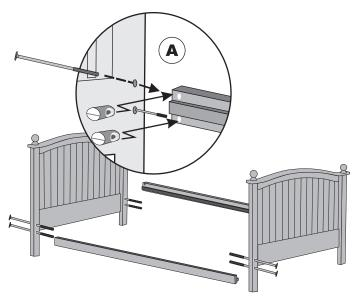
1) Attach foot board and head board to side rails. Insert barrel nuts into side rails. Insert 110mm bolts through end boards and into barrel nuts (See Diagram A).
