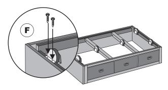
8) Attach casters to bottom of bed using two screws for each caster (See Diagram F). Notice that casters are located on the inside of each rail.
