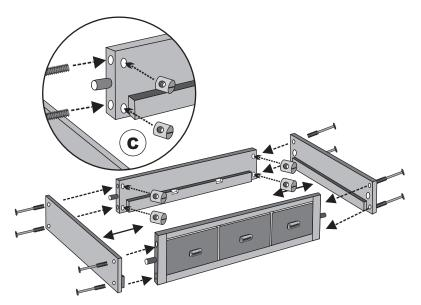
3) Attach the two lower bed end panels to the front and back panels. Use the 60 mm bolts and barrel nuts as shown in the diagram.(See Diagrams C).
