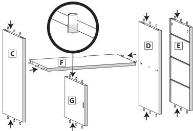
3) Place panel **D** on soft surface and locate panel **F**. Attach each panel so the finished edges are on the same side. Insert the pins into the corresponding holes in panel **F**. Secure panels by inserting one camlock into each of two corresponding holes on panel **F**. Turn each camlock clockwise about 1/4 turn or until gap between panels is gone. Do not over-tighten, it will damage the material.
